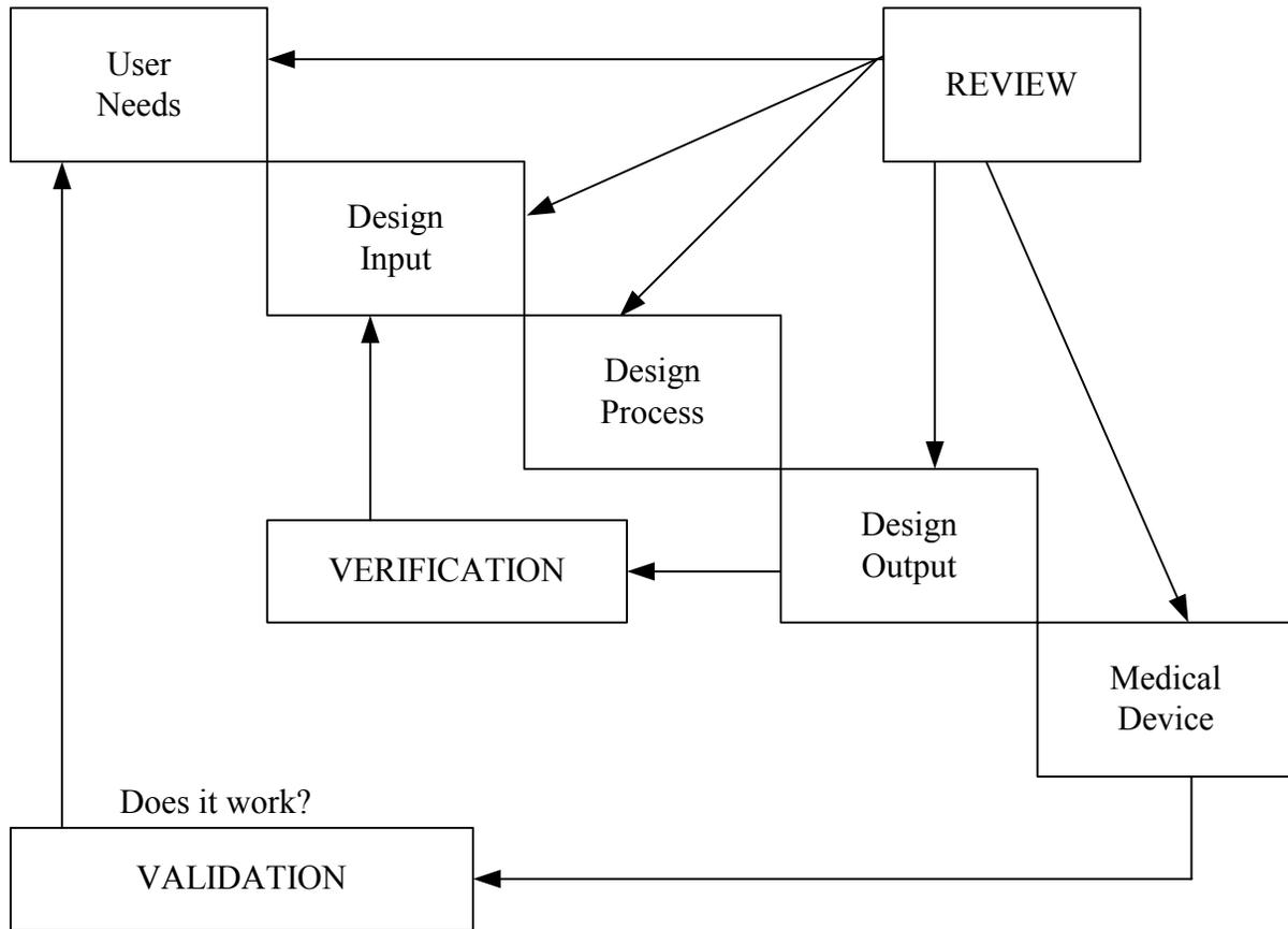
**Figure 1. Design Acceptance.** Adapted from the Federal Register: Part VII Dept. of Health and Human Services, FDA. 21 CFR Parts 808, 812, and 820. Rules and Regulations. October 7, 1996;61(195):52222–52601.
